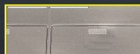
Figure 11. Photograph showing part of one pixel of the BUG array in detail. The TES sensor with its surrounding "Zebra" normal metal layer can be seen at the top center of the pixel.
